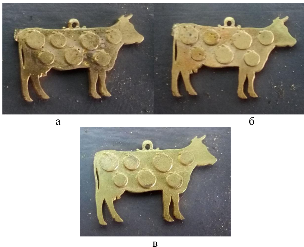
Figure 2. Castings made in molds with different temperatures: A - 500 °C; B - 550 °C; B - 640 °C
