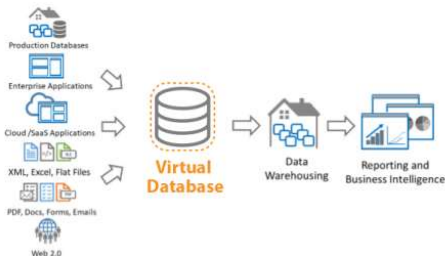
Fig .5. Database caching in Astera Data Virtualization
